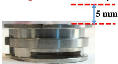
**Notice:** The **minimal** sample size should be **3 mm x 3 mm for XPS** and **5 mm x 5 mm for UPS** (UV beam size at stage is ~ 4 mm x 4 mm).
