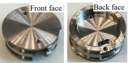
2) **60 mm** large sample holder for **as-is** sample analysis. This holder is good for large samples or more small samples. The three-hole metal mask can be used to ground and fix samples.
