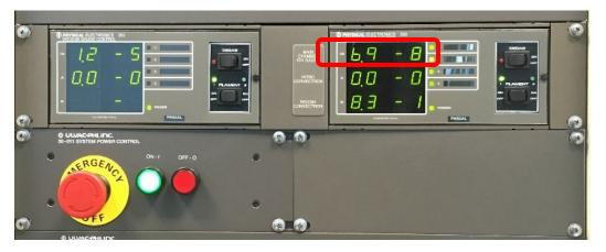
Check the "HV" high voltage LED light as highlighted in the picture below on the 11-425 E-BEAM SUPPLY box as highlighted below and make sure is ON in green. If the LED light is off, stop sample preparation and report to manager immediately.
