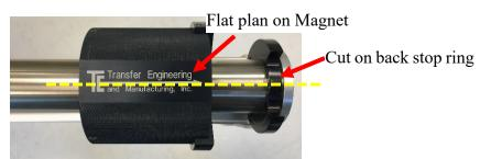
8) Grab the magnet with the right-hand thumb placed on the left side of magnet and **slowly** move toward main chamber until finger touches the stopper ring as show below.
