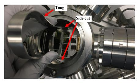
b) Make sure from the top-view below that the **scratched straight line** or the **flat cut** (new 60 mm sample holder) on the sample holder is on the right side (away from the
