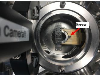
9) **Fully** retract the transfer arm with the magnet and let the flat plane face upward. Make sure the flat surface aligns the open cut on the back stop ring as highlighted by the dashed line below:
