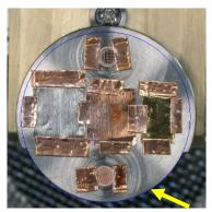
holder photo and make sure the **blue circle** aligns well with the **bottom half** (smaller circular part) of the **25 mm** sample holder. If not, contact lab manager. For **60mm** and **Angle-4 position** holder, the blue circle/rectangle should match the entire holder.
