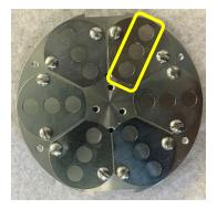
3) Angle-4 position sample holder. This holder is for Angle Resolved (AR) XPS/UPS.
