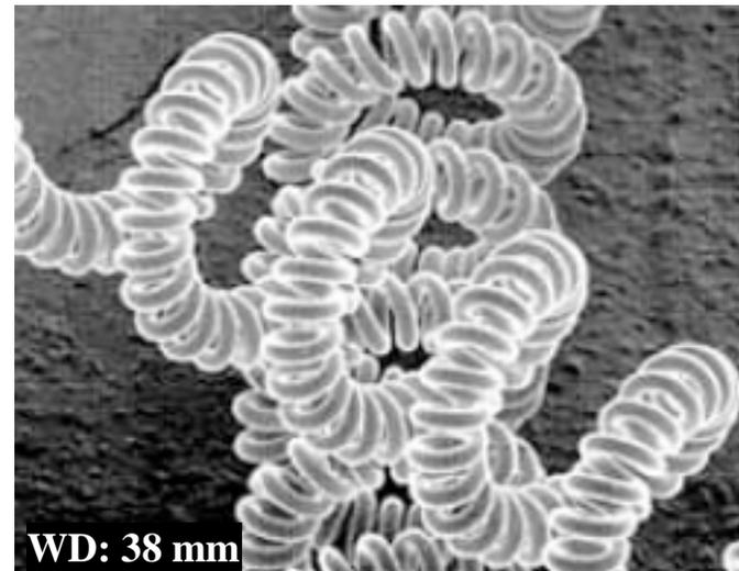
**Working Distance:** the distance between the bottom of the objective lens and the specimen
